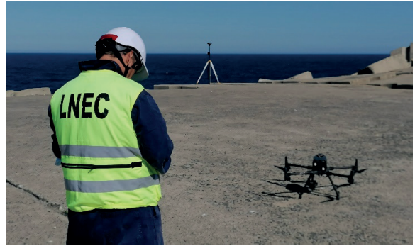
Figure 14. UAV operator preparing a flight on the Sines west breakwater; the RTK GNSS base antenna is visible at the top of the image
