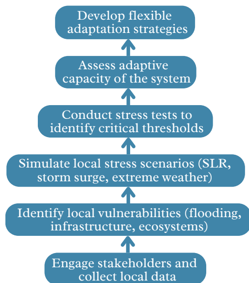
Figure 3. Bottom-up climate stress-testing framework applied to a coastal city.
