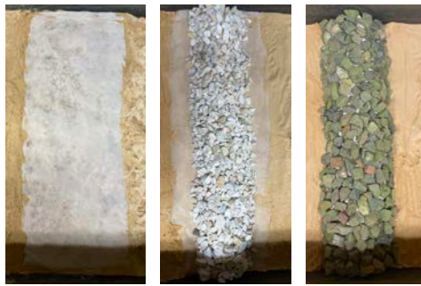
Figure 4: Initial rubble mound profile in the S test with photos depicting the placement sequence of filter (left), core (middle), and single armor layer (right) (green stone in Table 1).
