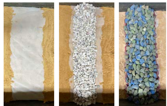
Figure 3: Initial rubble mound profile in the D test with photos depicting the placement sequence of filter (left), core (middle), and double armor layer (right) (green and blue combined in Table 1).
