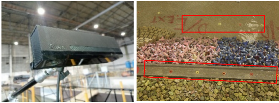
Figure 5. (a) Kinect position sensor; (b) ground control points
